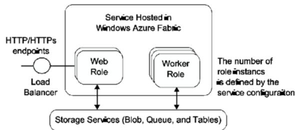
Figure 2. Architecture of a typical Azure application
