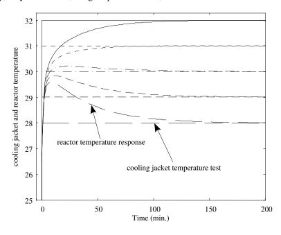
Figure 1. Batch reactor identification tests for different step changes in the cooling jacket temperature.
