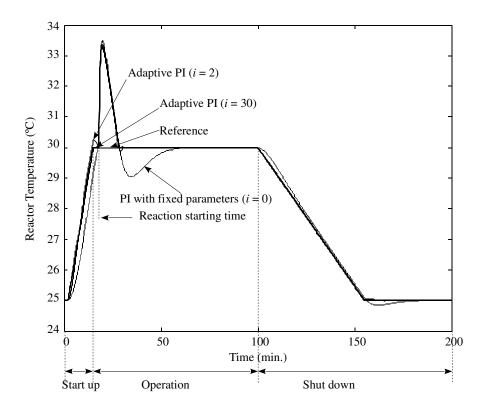
Figure 6. Controlled temperature inside the batch reactor when traditional feedback and adaptive feedback based-ILC are implemented.
