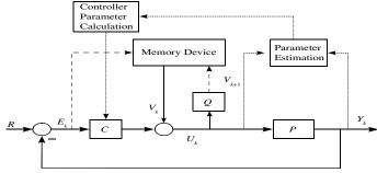
Figure 2. Schematic diagram of STR combined with feedback-based ILC. Here, continuous lines denote the signals used during the *k*-th trail, dashed lines denote signals will be used in the next iteration and doted lines belong to STR scheme.
