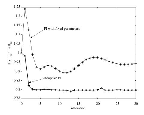
Figure 9. Ratio between  $||e||_{2,i}$  and  $||e||_{2,0}$ . Notice that,  $||e||_{2,i}$  is approximately reduced in a 20% for  $i \ge 3$  with respect to  $||e||_{2,0}$ . In addition, the  $l_2$ -norm could not be further reduced because of the saturation of the manipulated variable.
