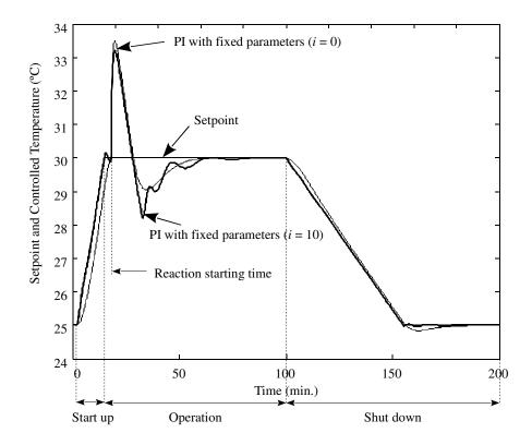
Figure 5. Setpoint and controlled temperature for iteration 0 (traditional feedback) and 10 (Feedback-based ILC) with limit in the manipulated variable.
