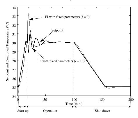
Figure 4. Setpoint and controlled temperature for iteration 0 (traditional feedback) and 10 when the manipulated variable is unbounded.
