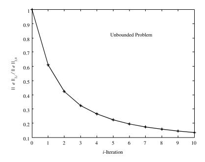
Figure 3. Ratio between  $\|e\|_{2,i}$  and  $\|e\|_{2,0}$  vs. *i*-trail when the feedback-base ILC is implemented with an unbounded manipulated variable.
