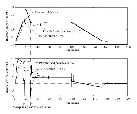
Figure 8. Temperature reaction response and manipulated variable for the traditional feedback and adaptive feedback based-ILC during the second iteration.
