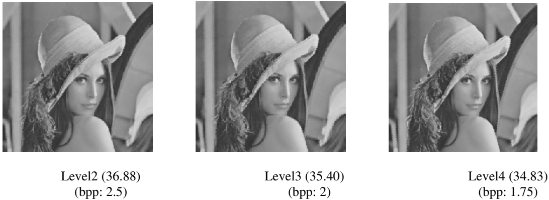
Figure 2: Comparison of reconstructed Images with the AMBTC and the Proposed Methods
