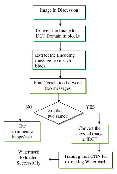
Figure 6 Process of watermark extraction
