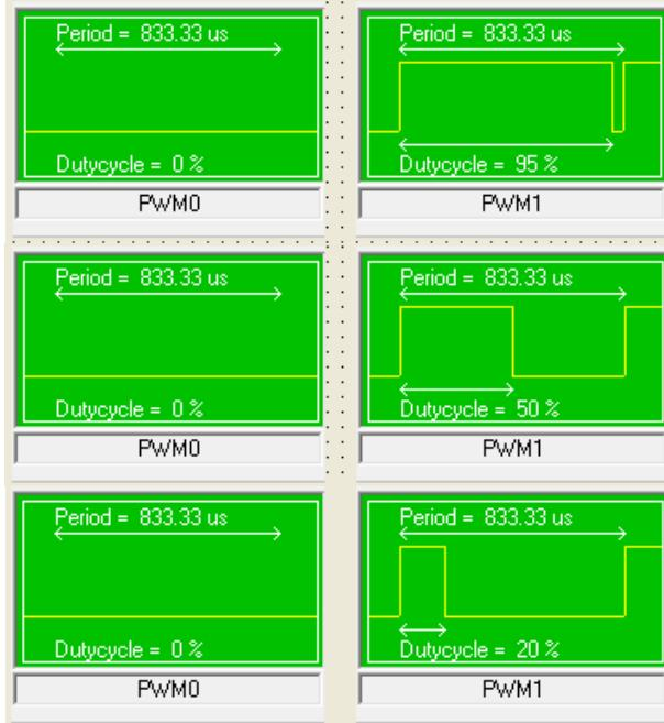
Fig:3: PWM for Clockwise Rotation at 20 MHz Crystal
