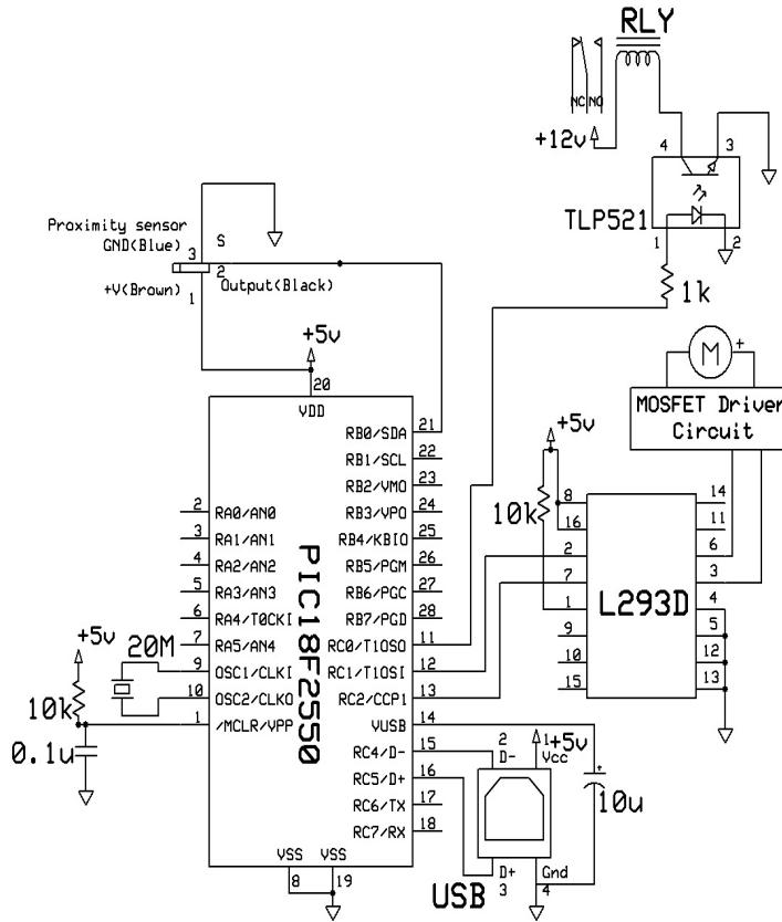
Fig: 5: Schematic Diagram of Implemented Circuit
