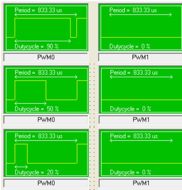
Fig:4: PWM for Anti-Clockwise Rotation at 20 MHz Crystal
