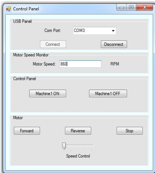
Fig:2: Designed GUI
