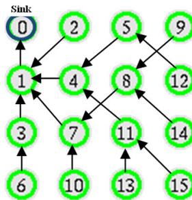
Figure 1. Simulated network tree topology.
