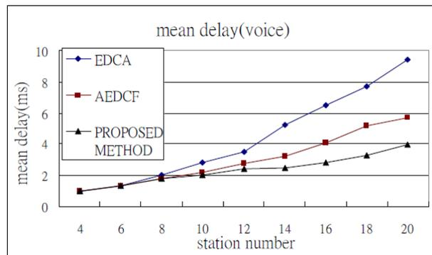
Figure 10 The mean delay of Voice
