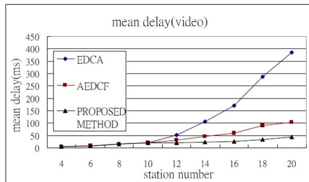
Figure 11 The mean delay of Video
