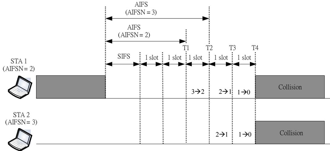
Figure 2 The collision occurs among stations with different AIFSNs
