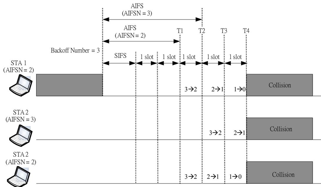
Figure 1 The collision occurs among stations with the same AIFSN or the same back-off counter
