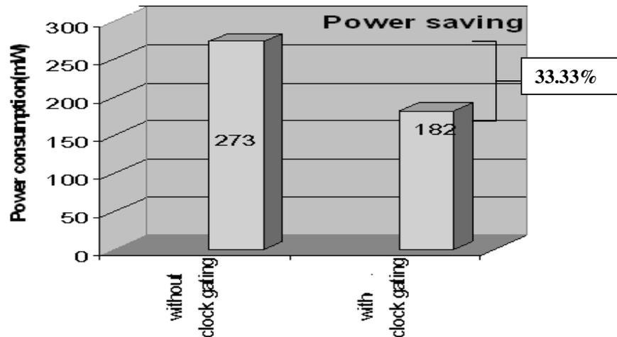
Figure.11 Comparison of Power Consumed without and with Clock Gating
