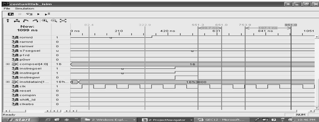
Figure.6 Control Unit Simulation Results (contd...)
