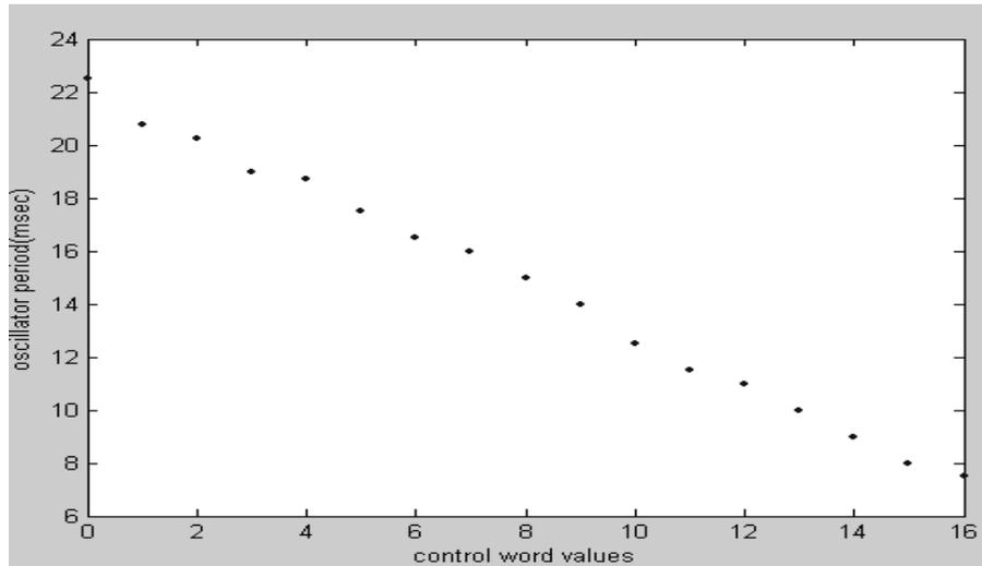
Figure.3 Oscillator Cycle Time vs. Control Word Value
