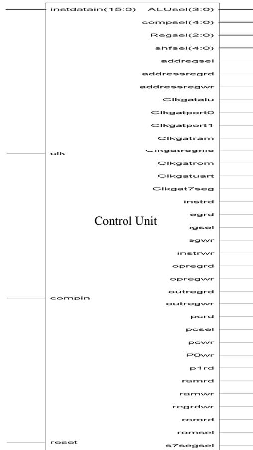
Figure.5 Signals of Control Unit
