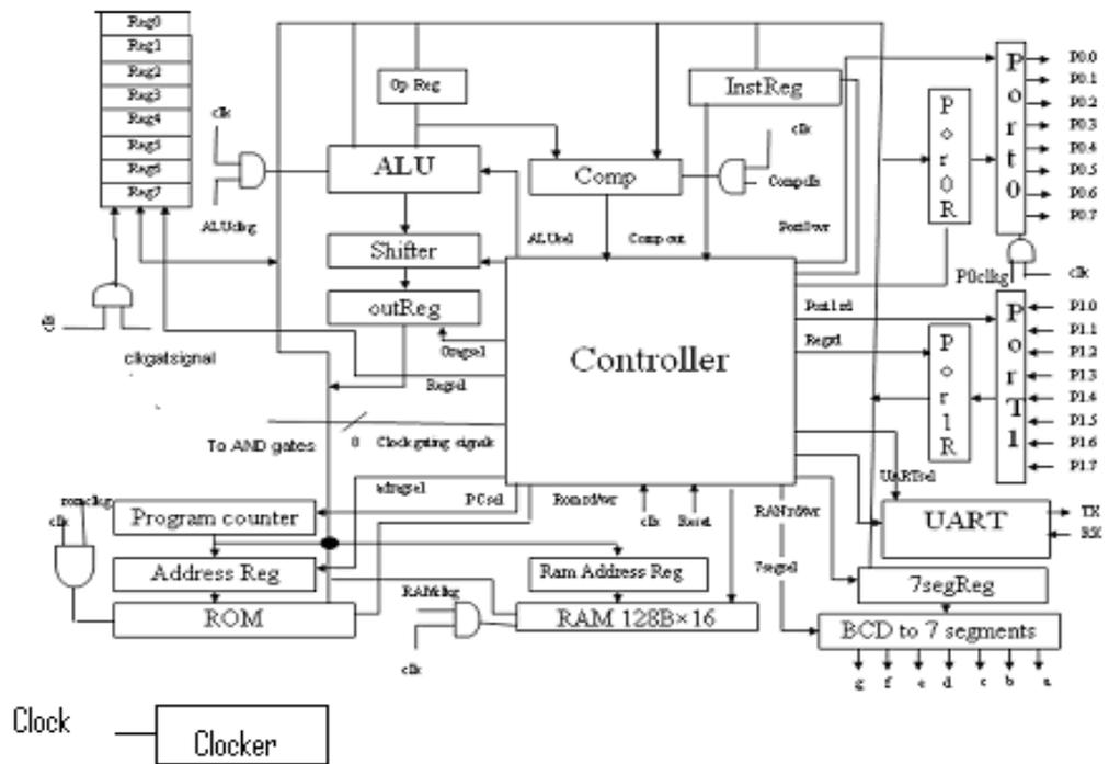
Figure.1 Architecture of Programmable Embedded Controller
