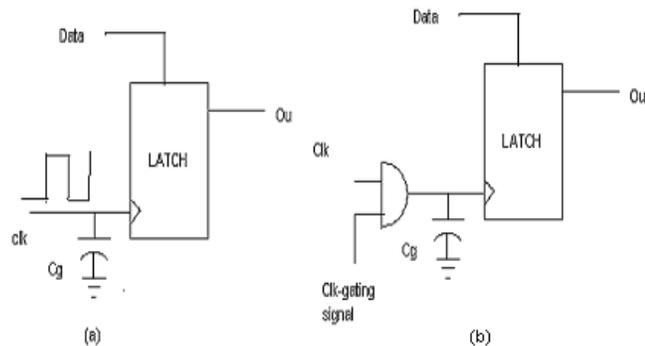
Figure.4 Schematic of Latch Element (a) without clock gating (b) with clock gating
