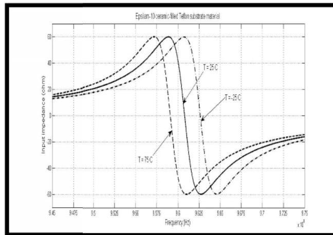
Figure. 26. Imaginary part of the input impedance as a function of frequency at different temperatures 75, 25 and -25 °C and radius of curvature 50 mm.
