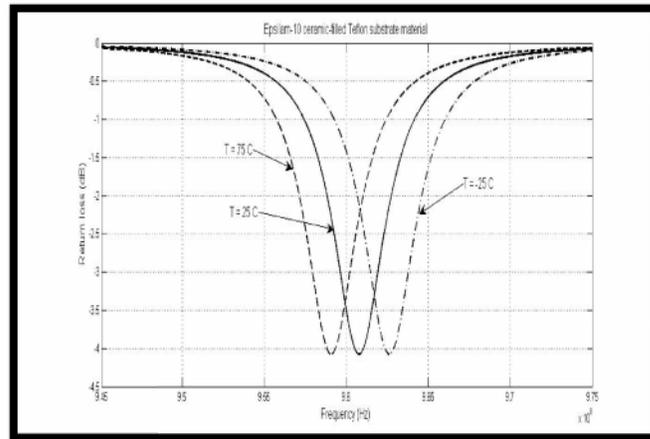
Figure. 28. Return loss (S11) as a function of frequency at different temperatures 75, 25 and -25 °C and radius of curvature 50 mm.
