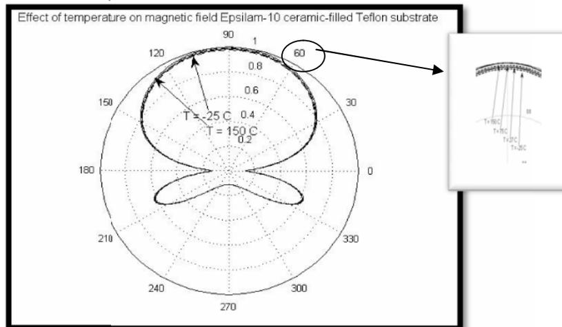
Figure. 30. Normalized magnetic field for different temperatures 150, 75, 27 and -25 °C. at  $\theta = 0:2$  and  $\phi = 0^0$  and radius of curvature 50 mm.
