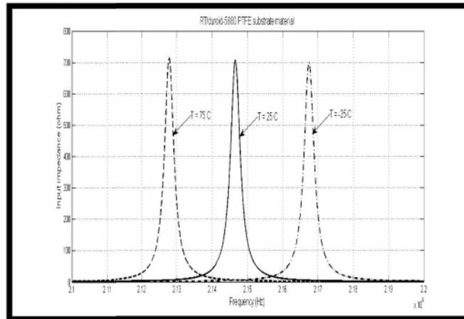
Figure. 9. Real part of the input impedance as a function of frequency at different temperatures 75, 27 and -25 °C and radius of curvature 50 mm.
