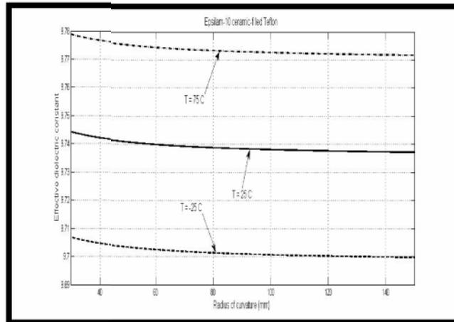
Figure. 23. Effective dielectric constant versus radius of curvature for cylindrical-rectangular and flat microstrip printed antenna at different temperatures 75, 25 and -25 °C.
