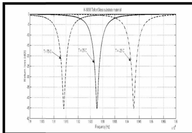
Figure. 20. Return loss (S11) as a function of frequency at different temperatures 75, 25 and -25 °C and radius of curvature 50 mm.
