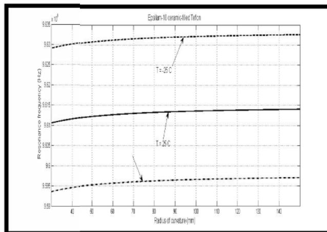
Figure. 24. Resonance frequency versus radius of curvature for cylindrical-rectangular and flat microstrip antenna for TM<sub>01</sub> at different temperatures 75, 25 and -25 °C.
