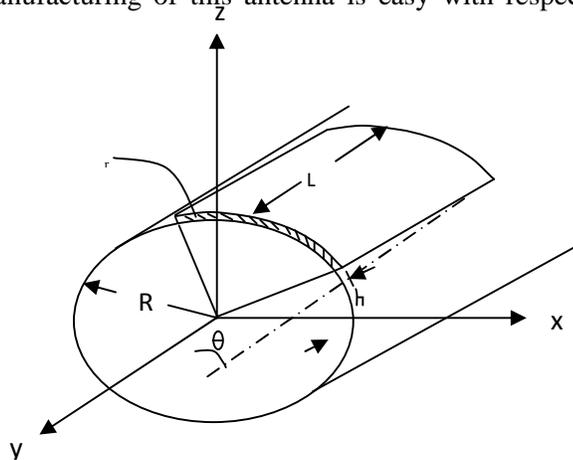
Figure 4: Geometry of cylindrical-rectangular patch antenna
