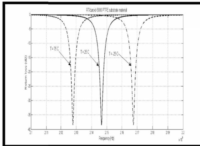
Figure. 12. Return loss (S11) as a function of frequency at different temperatures 75, 25 and -25 °C and radius of curvature 50 mm.
