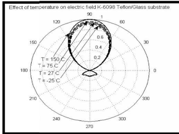
Figure. 21. Normalized electric field for different temperatures 150, 75, 27 and -25 °C. at  $\theta=0:2$  and  $\phi=0^0$  and radius of curvature 50 mm.
