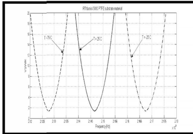
Figure. 11. VSWR versus frequency at different temperatures 75, 25 and -25 °C and radius of curvature 50 mm.
