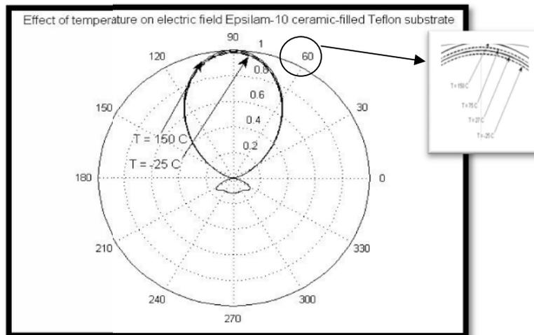
Figure. 29. Normalized electric field for different temperatures 150, 75, 27 and -25 °C. at  $\theta = 0:2$  and  $\phi = 0^0$  and radius of curvature 50 mm.
