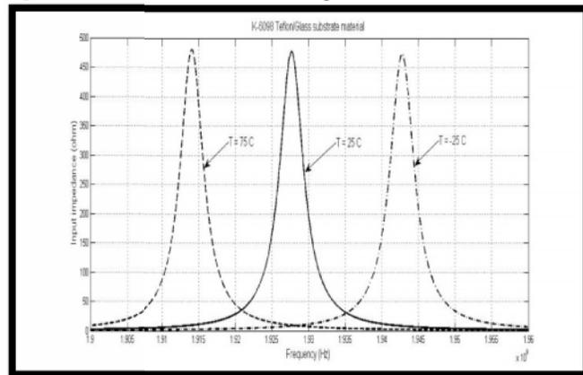
Figure. 17. Real part of the input impedance as a function of frequency at different temperatures 75, 25 and -25 °C and radius of curvature 50 mm.
