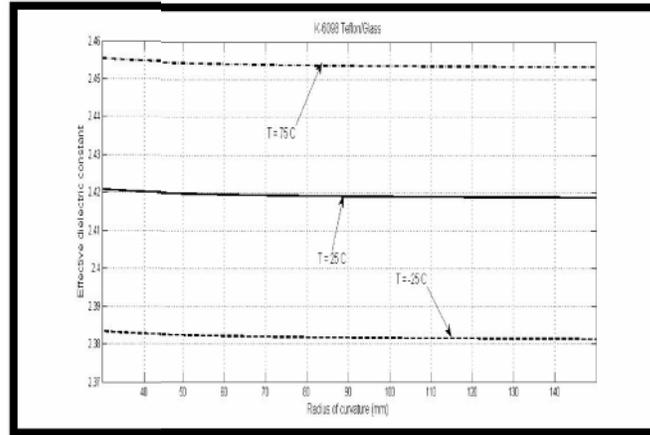
Figure. 15. Effective dielectric constant versus radius of curvature for cylindrical-rectangular and flat microstrip printed antenna at different temperatures 75, 25 and -25 °C.
