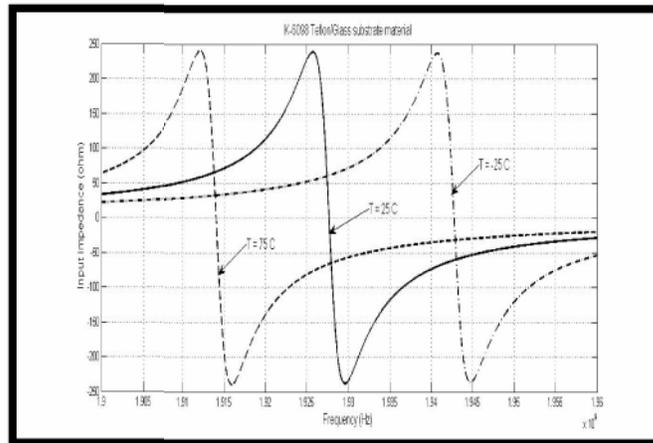
Figure. 18. Imaginary part of the input impedance as a function of frequency at different temperatures 75, 25 and -25 °C and radius of curvature 50 mm.
