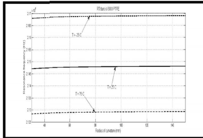
Figure. 8. Resonance frequency versus radius of curvature for cylindrical-rectangular and a flat microstrip printed antenna at different temperatures 75, 25 and -25 °C.
