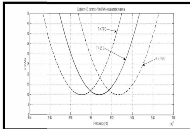
Figure. 27. VSWR versus frequency at different temperatures 75, 25 and -25 °C and radius of curvature 50 mm.
