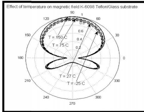
Figure. 22. Normalized magnetic field for different temperatures 150, 75, 27 and -25 °C. at  $\theta=0:2$  and  $\phi=0^0$  and radius of curvature 50 mm.
