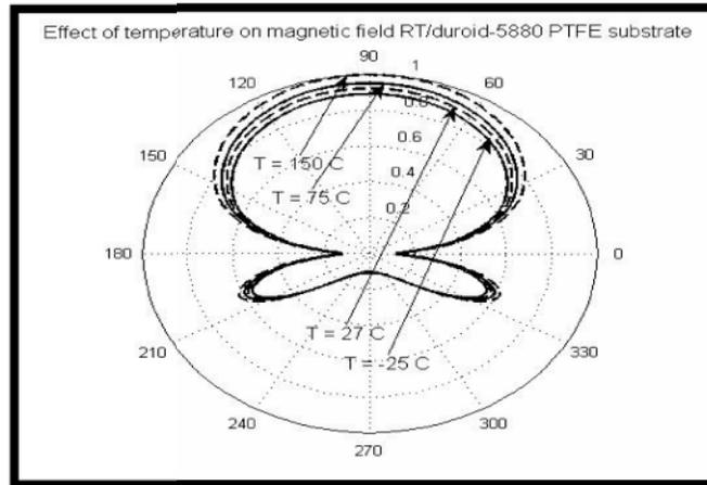
Figure. 14. Normalized magnetic field for different temperatures 150, 75, 27 and  $-25^{\circ}\text{C}$ . at  $\theta=0:2$  and  $\phi=0^{\circ}$  and radius of curvature 50 mm.
