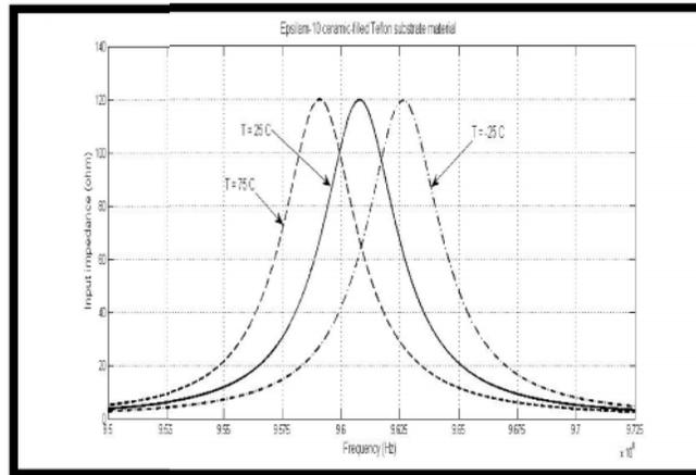
Figure. 25. Real part of the input impedance as a function of frequency at different temperatures 75, 25 and -25 °C and radius of curvature 50 mm.
