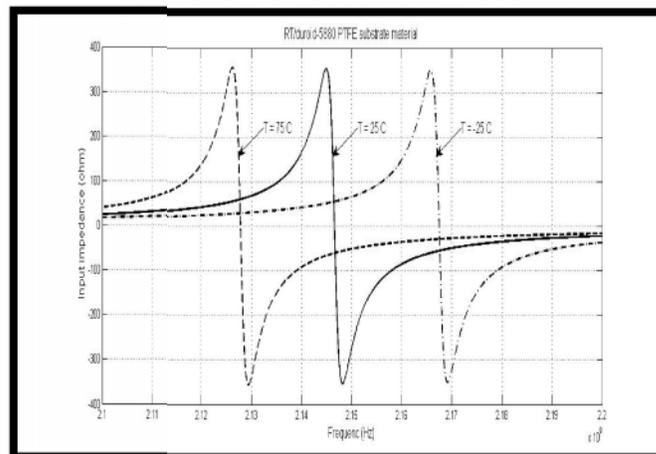
Figure. 10. Imaginary part of the input impedance as a function of frequency at different temperatures 75, 25 and -25 °C and radius of curvature 50 mm.
