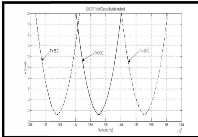
Figure. 19. VSWR versus frequency at different temperatures 75, 25 and -25 °C and radius of curvature 50 mm.
