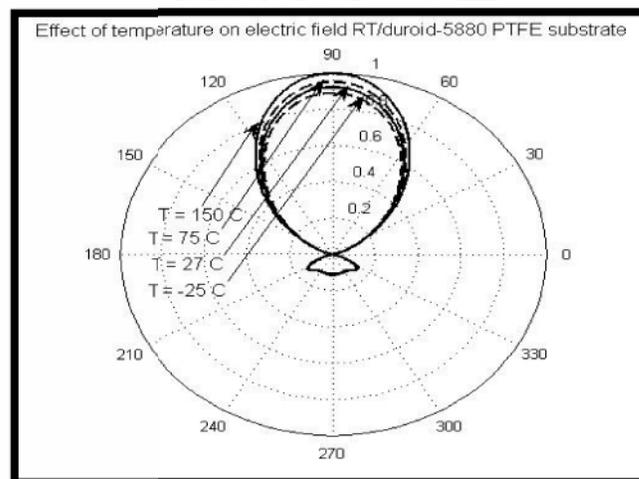
Figure. 13. Normalized electric field for different temperatures 150, 75, 27 and -25 °C. at  $\theta=0^\circ$  and  $\theta=180^\circ$  and radius of curvature 50 mm.
