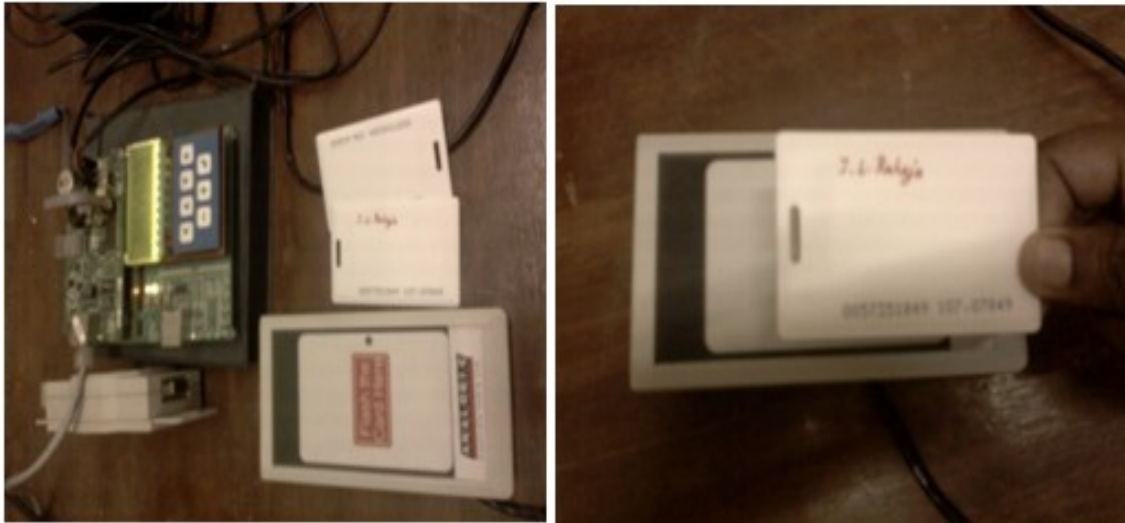
Figure 10. GECS Client system hardware with RFID reader, tag and microprocessor based NIC unit and a RF Tag flashing in front of reader
