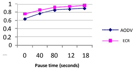
Figure3. Packet Delivery Fraction. Number of Nodes: 40
