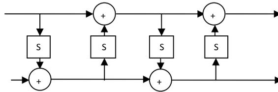
Figure 2. Lifting scheme.
