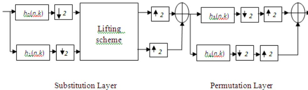
Figure 3. One Round Filter Bank Encryption cipher.
