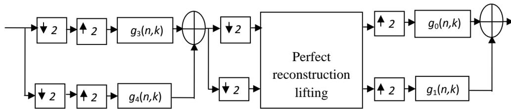
Figure 5. One Round filter bank cipher decryption System.
