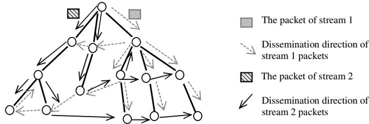
Figure 1. An example of a multitree based hybrid overlay network.
