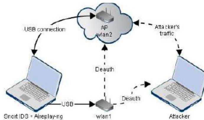
Figure 3. Final topology – Scenario: Running Snort on wireless router
