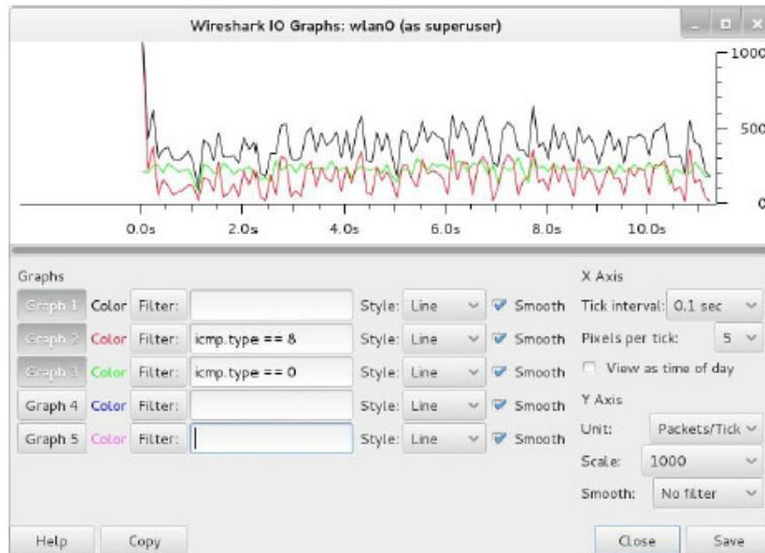
Figure 4. Wireshark statistics of ICMP flood attack
