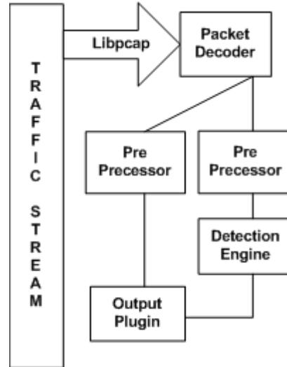
Figure 4. Snort component data-flow
