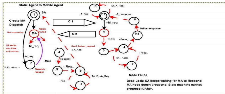
Figure 10: Deadlock error in Node Monitoring protocol
