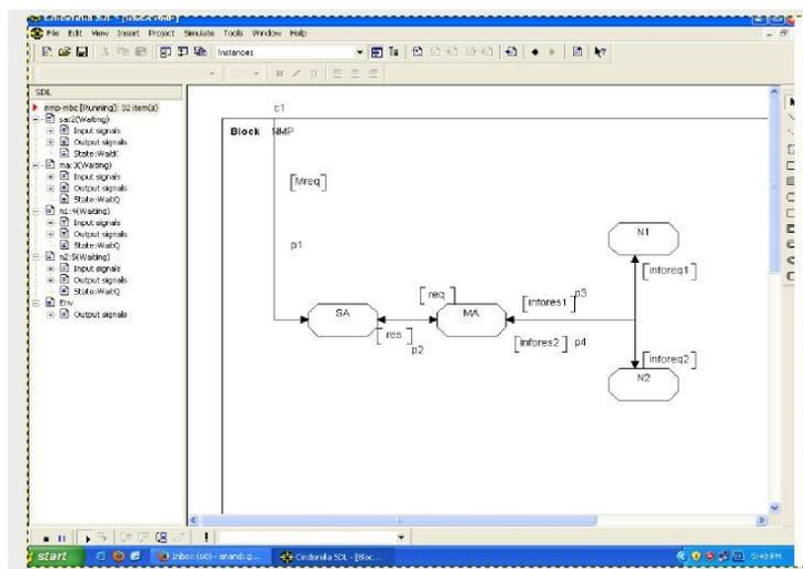
Figure 3: Blocks of Node Monitoring protocol using SDL
