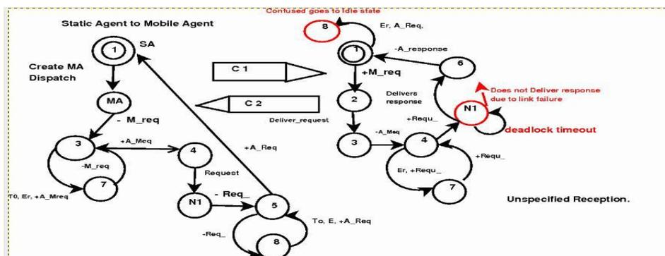
Figure 12: Unexpected State error in NMP
