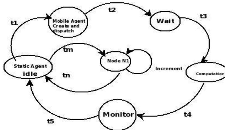
Figure 1: Formal FSM specification of NMP
