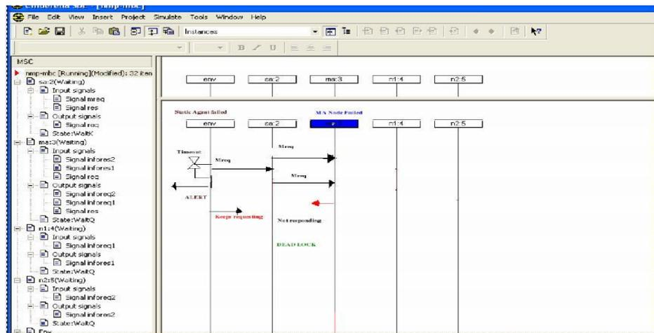
Figure 11: Message Sequence chart showing Dead Lock error in NMP
