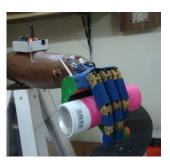
Fig.7. The FFRH grasping a variety of objects.(Bulb, Bottle, Ball, Tin, and Duster).
