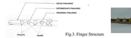
For practical reasons, epoxy is selected as the material for the plates (fingers) since it is strong, rigid, lightweight, relatively in expensive, and easy to machine. We also choose epoxy 95
