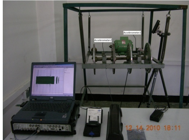
Figure16.A laboratory scale experimental double four-bar crank-slider mechanism setup
