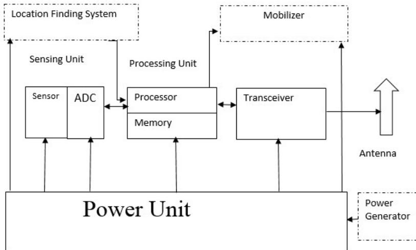
Figure: 2 Block diagram sensor networks
