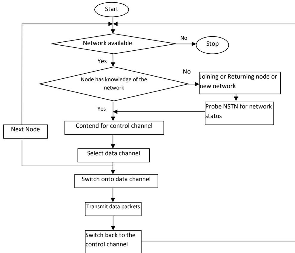
Fig 2. The implementation of the network infrastructure in the Cyclic Scheduling Algorithm
