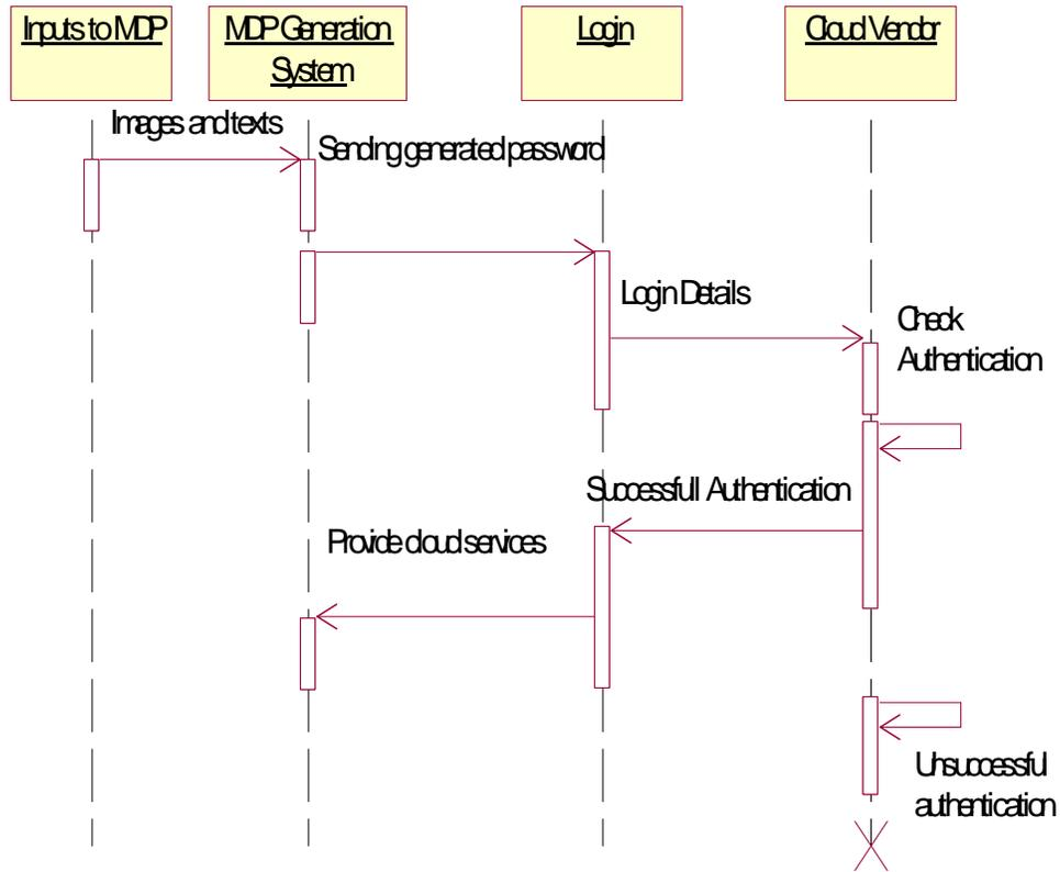
Fig. 3: Sequence diagram to generate multi-dimensional password
