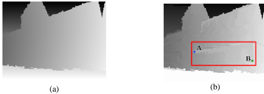
Figure 6. Depth hypothesis generation. (a) local depth hypothesis H_{local} , (b) initial depth map D_{init} .
