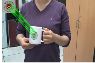
Figure 3. Results of SIFT matching of a logo template and an input frame F_n .
