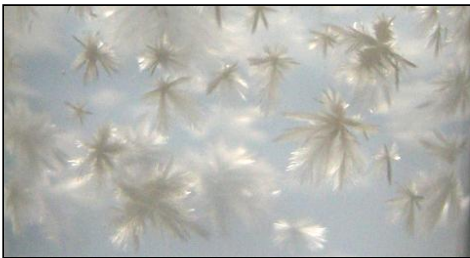
Figure 4 Magnified view of multi-branching tree-like form (fractal with center) dendrite crystals of lead iodate
