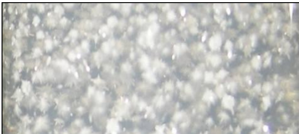
Figure 3 Magnified view of spiky spherulites crystals of lead iodate
