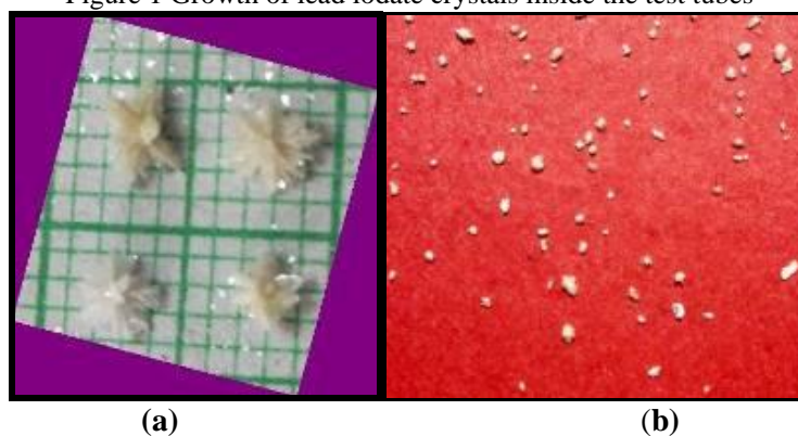
Figure 2 Lead iodate crystals outside the test tubes (a) fractal dendrite aggregate crystals and (b) spiky spherulitic and platelets crystals
