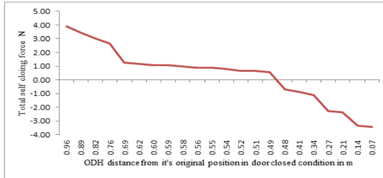
Figure 6. Total self-closing forces due to hinge inclination Vs. Door Opening distance from its original
