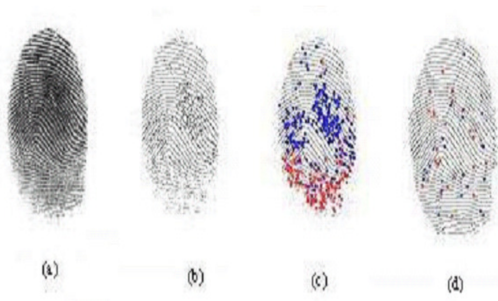
Figure23. Image enhancement result, (a) original image 101_2.tif, (b) thinned image with out enhancement (c) minutiae point detected with out enhancement and (d) minutia point detected with image fingerprint enhancement.
