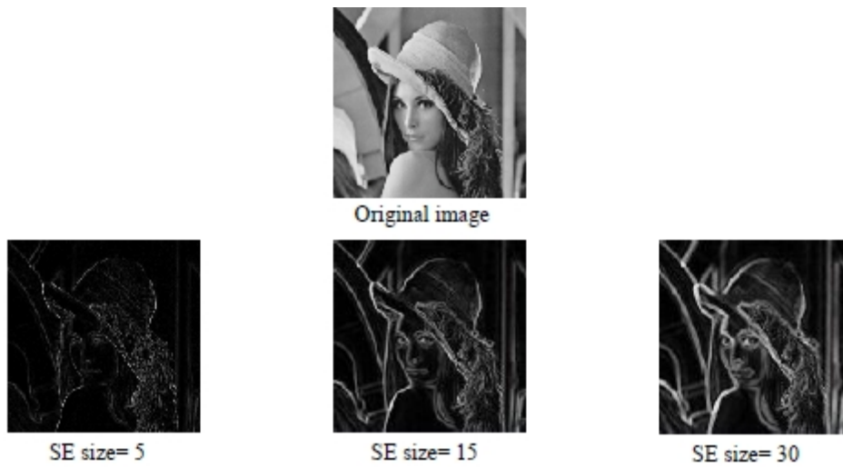
Figure (4.6) Apply boundary extraction algorithm on grayscale image with SE type = diamond
