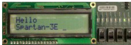
Figure 8. Display of LED and LCD at FPGA Spartan 3E Starter Kit [4]
