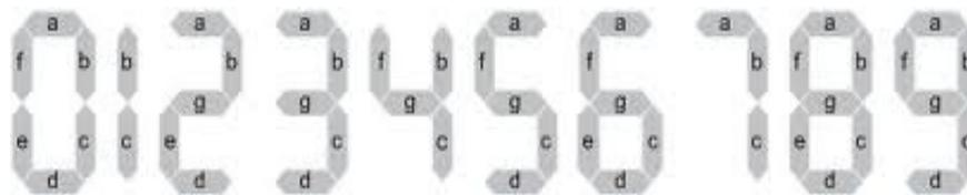
Fig.3: Display of numbers using seven segments
