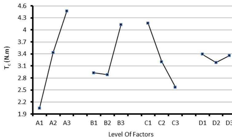
Figure3. Main factor effects on peak to peak value of cogging torque
