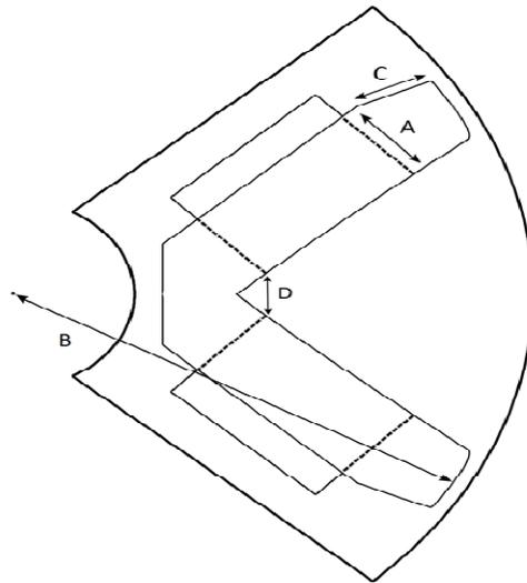
Figure1. Rotor configuration of v-type IPM motor.
