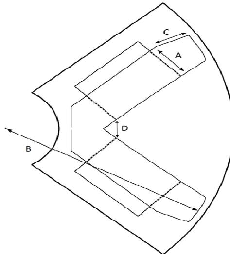
Figure1. Rotor configuration of v-type IPM motor.
