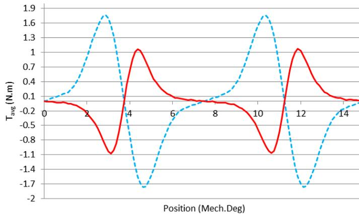
Figure6. Cogging torque of initial design (blue line) and optimized design (red line)
