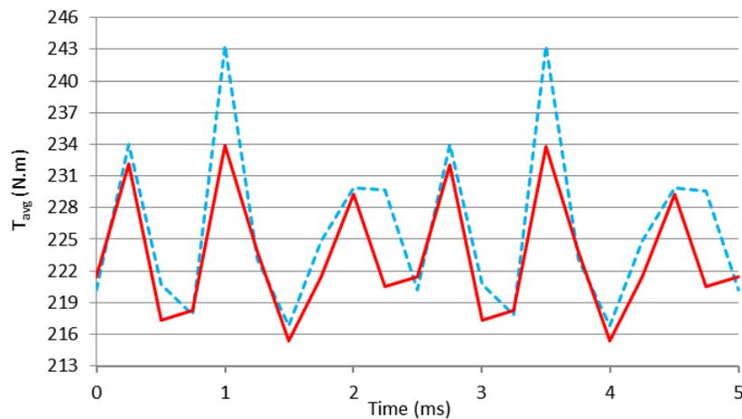
Figure5. Output torque of initial design (blue line) and optimized design (red line)
