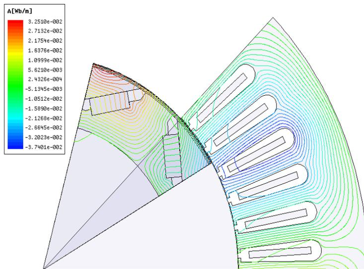
Figure4. Magnetic field distribution for IPM motor
