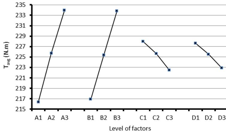
Figure2. Main factor effects on average torque
