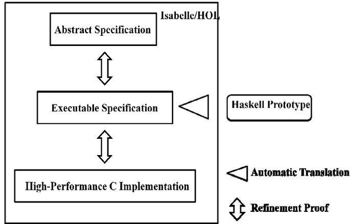
Figure 7. The refinement layers in the verification of seL4 [43]
