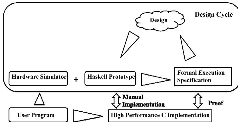
Figure 6. The seL4 design process [43]
