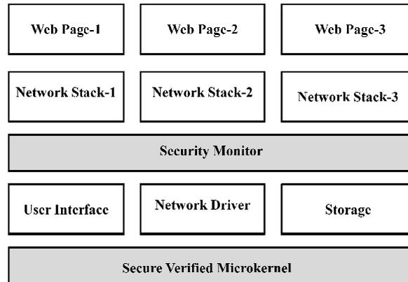
Figure 8. Secure web browser architecture. Components that belong to the TCB of the system are highlighted using grey shading[20]
