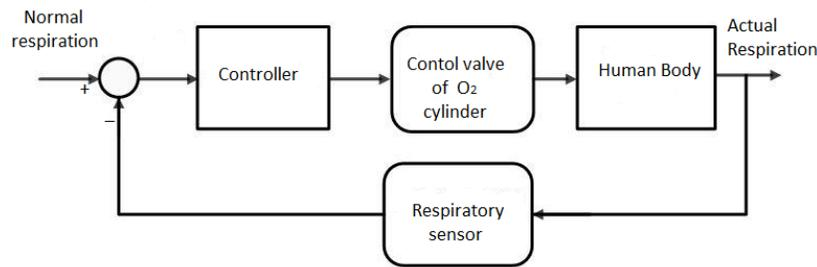
Figure 1: Closed Loop Control
