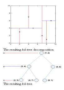
Let us consider some data points in a given plane. As sho wn in the above figure there are six data points in the plane. We can form a K-D tree for those data points by considering their x co-ordinate and y co-ordinate. The resulting K-D tree is as shown in the above[8].
