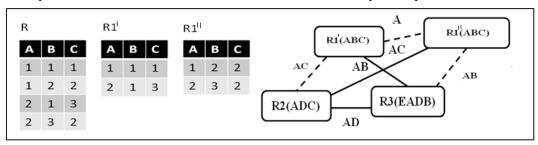
Figure 13. Removal of cycle using horizontal decomposition of a relation
