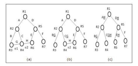
Figure 10. Removal of cycle using Attribute Addition Approach.
