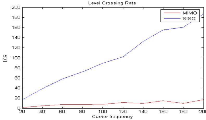
Fig 5a: LCR vs Carrier frequency with different channel practically
