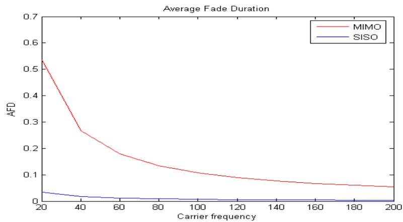
**Fig4b:AFD vs Carrier Frequency with different channel theoretically**
