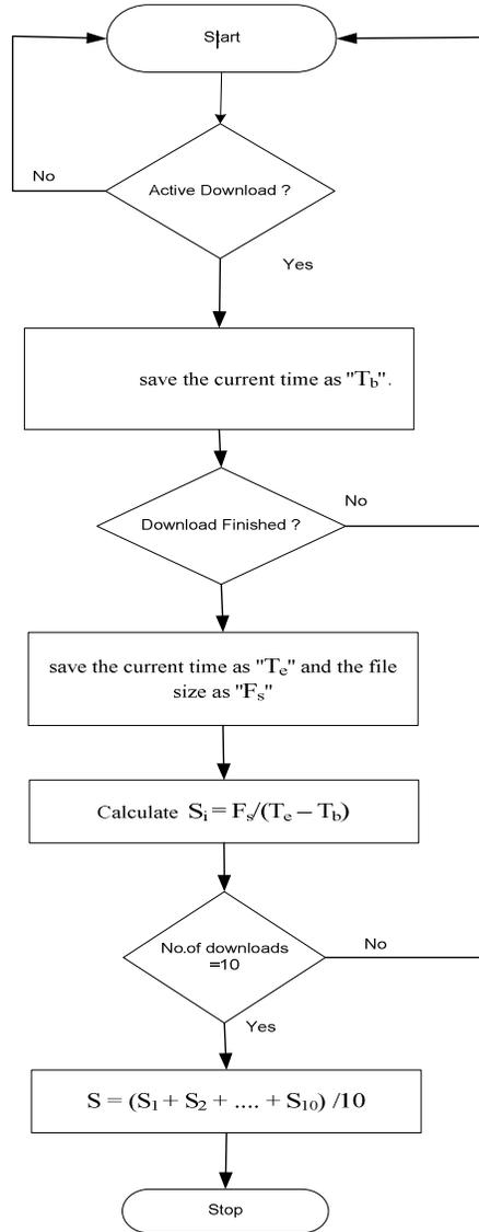
**Figure 2:** QMeter’s Bandwidth Calculation flowchart
