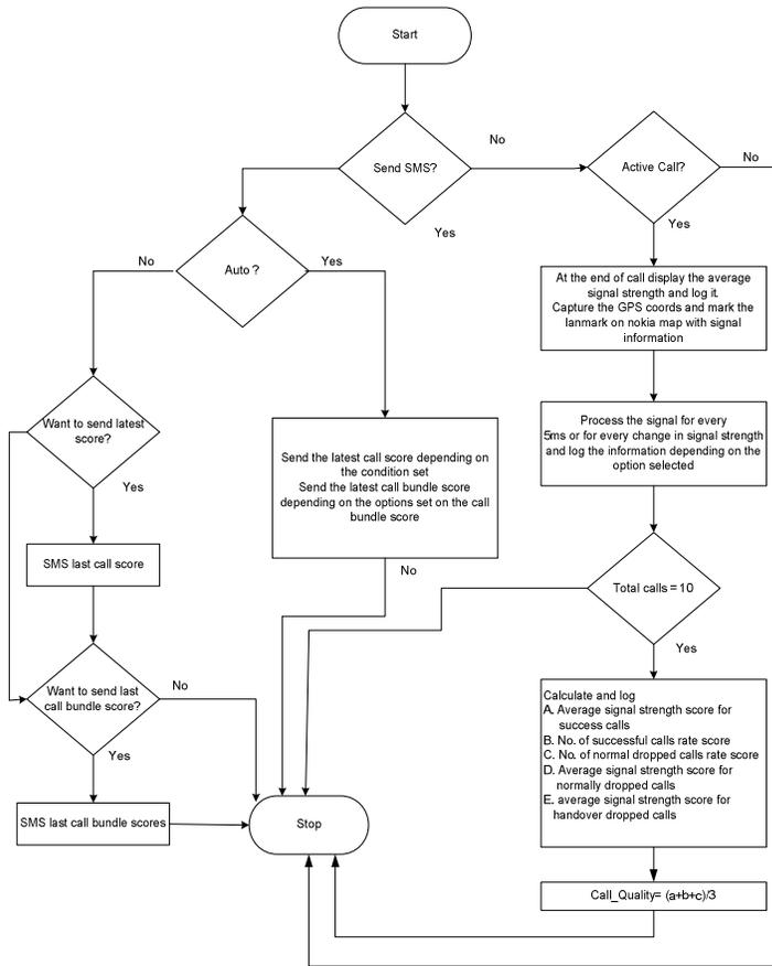
Figure 1: QMeter's Call Quality measurement flowchart
