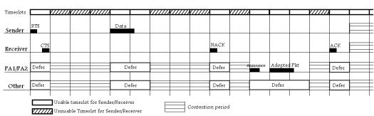
Figure 3. Slotted Packet Transmission
