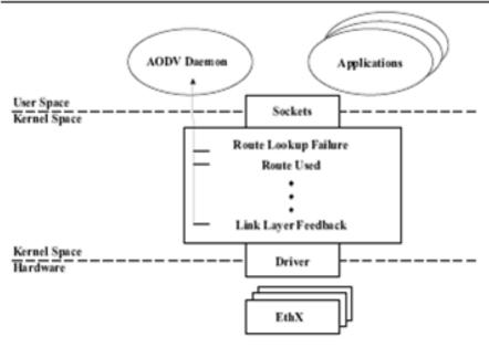
Figure 3. Kernal Modification Architecture
