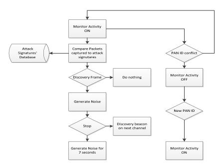
Figure 7. Intrusion Detection Algorithm
