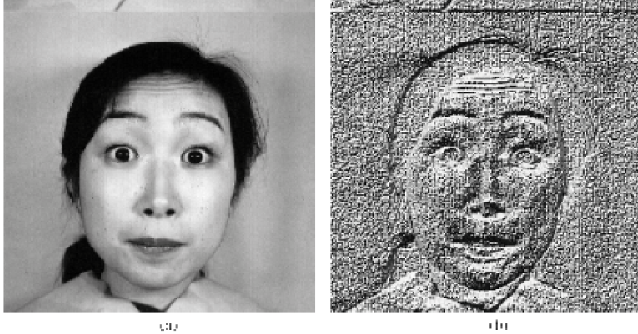
Fig. 3: Census Transformation of an image: (a) original image, and (b) CT image.
