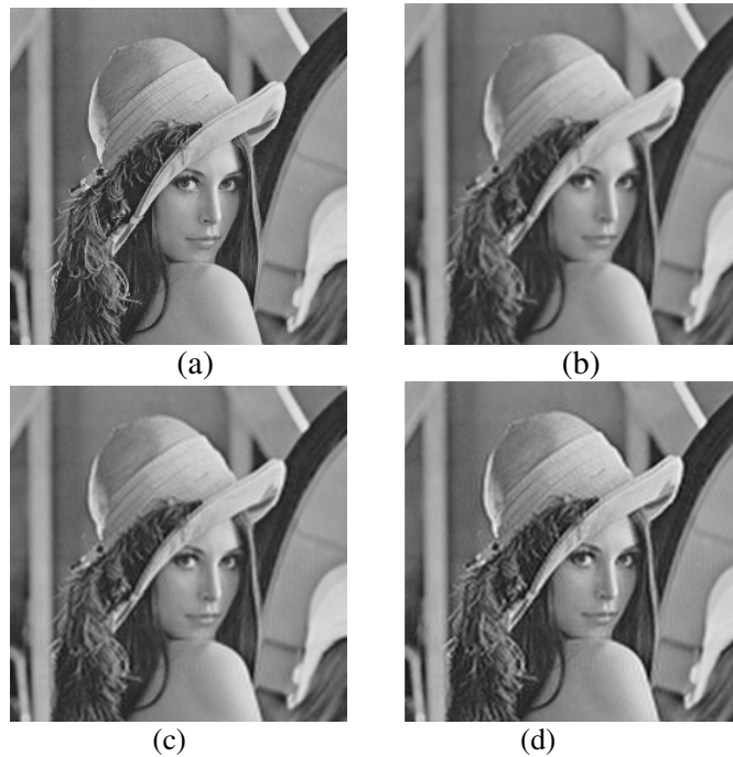
Fig.5: Subjective Evaluation of Lena using different Interpolation Techniques: (a) Source image (b) Bicubic method (c) DCT method (d) Proposed Method.
