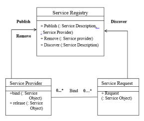
Figure 1. Service Oriented Architecture: Conceptual Model
