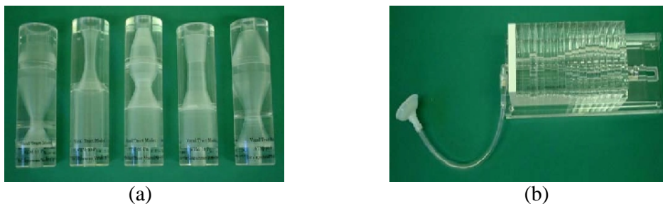
Figure.3 Physical model of the human vocal tract (a) cylinder model and (b) plate model [13].
