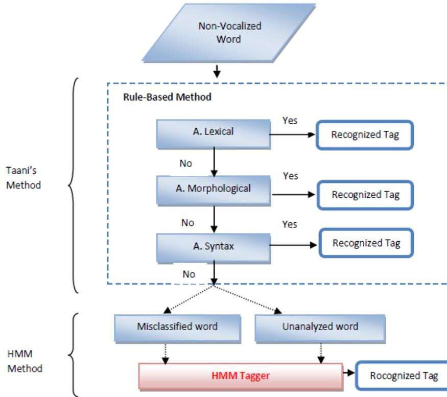
Figure2. Flowchart of the Proposed Arabic POS Tagger
