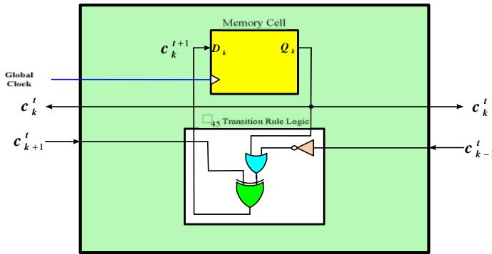
Figure 5-  $\square_{45}$  logic circuit realization with memory cell at spatial index  $k$ .
