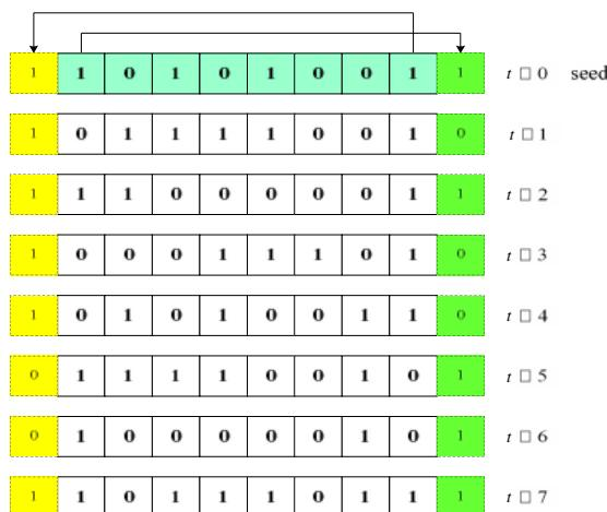
Figure 7- seven time-steps evolution of uniform periodic ECA with 8-cell span length using  $\square_{45}$ .
