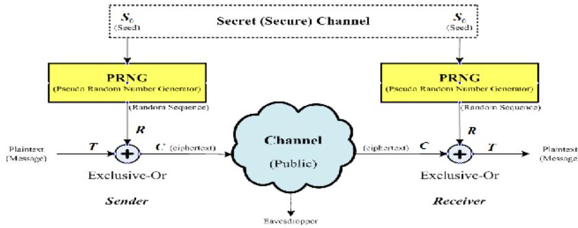
Figure 1. Typical Synchronous Stream Cipher.
