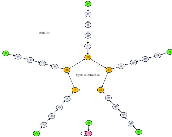
Figure 13- State Diagram of a periodic ECA running uniformly under rule  $\phi_{30}$  for  $K = 5$ .
