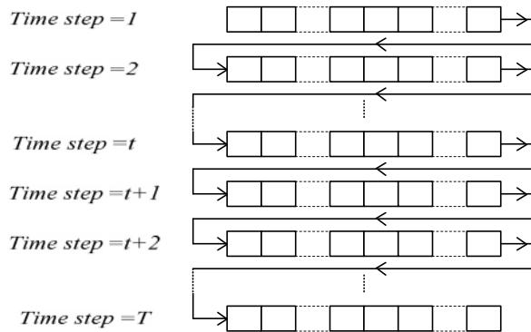
Figure 12 - Concatenation of the ECA output data stream by the output function  $\varphi$ .
