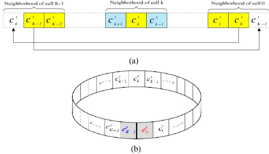
Figure 2- Illustration of periodic (circular) ECA configuration.
