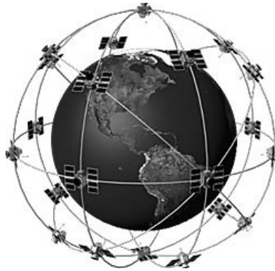
Figure 1. GPS consists of 24 satellites of which at least 5 can be seen from any point on the globe. [10]
