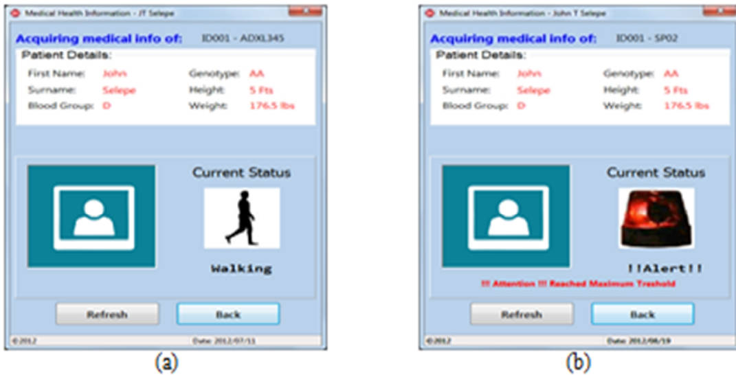
Figure 6. Screenshots of the CIN’s GUI showing (a) patient walking (ID – 3) on accelerometer monitoring and (b) an alert message in case of an emergency on pulse oximeter monitoring
