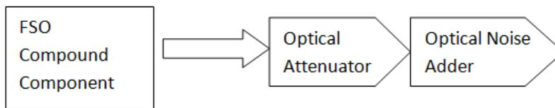
Figure.2. Simulation set-up for the FSO link
