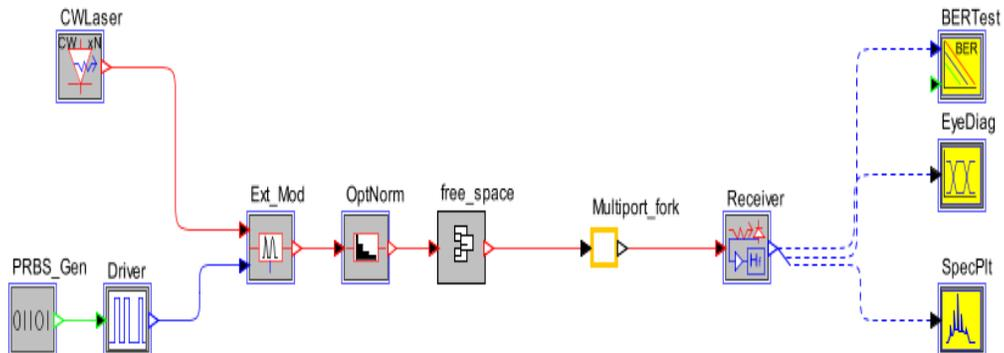
Figure.3. Simulation setup for FSO link
