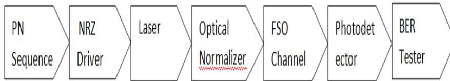
Figure.1. Block Diagram
