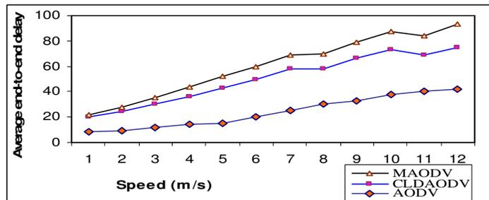
Figure 4(b). Average end-to-end delay versus speed(m/s) for MAODV, CLAODV and AODV.
