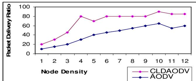
Figure 5(a). Packet delivery Ratio versus Node density for CLDAOV and AODV.
