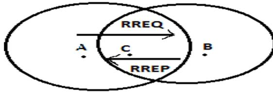
Figure 2. Route Reply failure due to low power nodes B, and C
