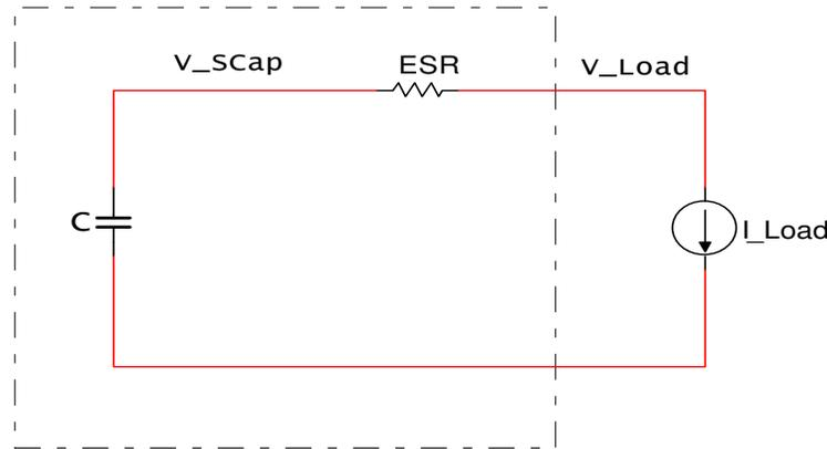
Figure 6. An ideal supercapacitor circuit model
